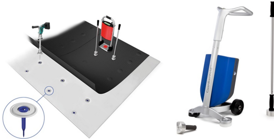
FIGURE 17: PRINCIPLE OF INDUCTION WELDING
