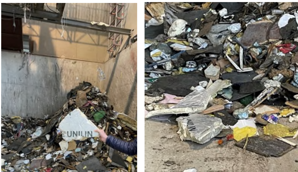
FIGURE 27: PU AMONG OTHER PLASTICS AND LIGHT MATERIAL AFTER SORTING
